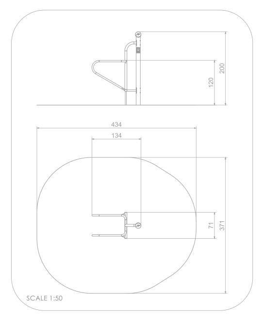
MATERIALS: SOLID CONSTRUCTION MADE OF BLACK STEEL S235JR, CLEANED IN THE SANDBLASTING PROCESS
