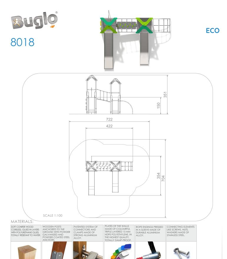
SUDES MADE OF STAINLESS STEEL AISI 304, METAL SHEET WITH A THICKNESS OF 2 MM FORMED IN A CNC TECHNIQUE. ANTI-SLIP ANTHRACITE 10MM HPL PLATFORM PLATE WITH A VERY HIGH RESISTANCE TO WEATHER CONDITIONS AND ATTRITION
